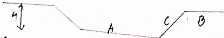
$$\text{length of bar } B_2 : A + B + C = 400 + 2 \times 230 - 2 \times 40 + (1.414 \times 4 - 4)$$
