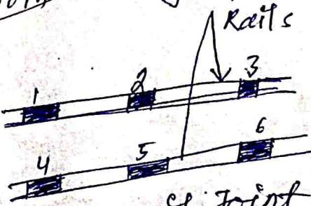
Even Joint: in this also the position of gear joint is the basis of its nomenclature, the joints of one gear track are directly opposite to the joints of other gear track.
